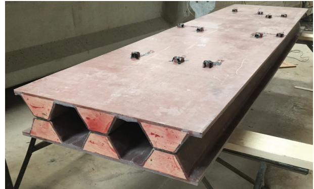
Photo of Composite Bridge Deck
